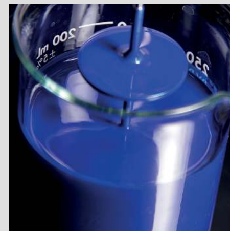
Paint and ink dispersion Maximizing the efficiency of the finishing process by dispersing and homogenizing difficult-to-disperse pigments.
