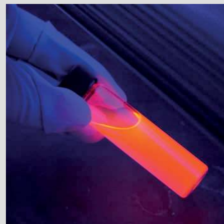
Luminescent material for display homogeneous dispersion of polymer resin and powder.
